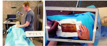
Figure 2. The surgeon views the operating field through a transparent display that shows the annotations generated by the expert. The annotations are integrated directly into the field of view of the surgeon. When the display is repositioned, the annotations remain anchored to the operating field entities that they describe.
