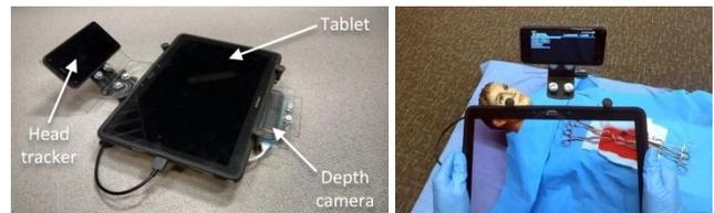
Figure 4. Left: hand-held, self-contained transparent display prototype built from tablet computer enhanced with on-board user head tracking and geometry acquisition accessories. Right: first test of transparent display in the surgical telementoring context. The accurate transparency effect provides visual continuity between the parts of the operating field seen directly and the parts seen through the display.
