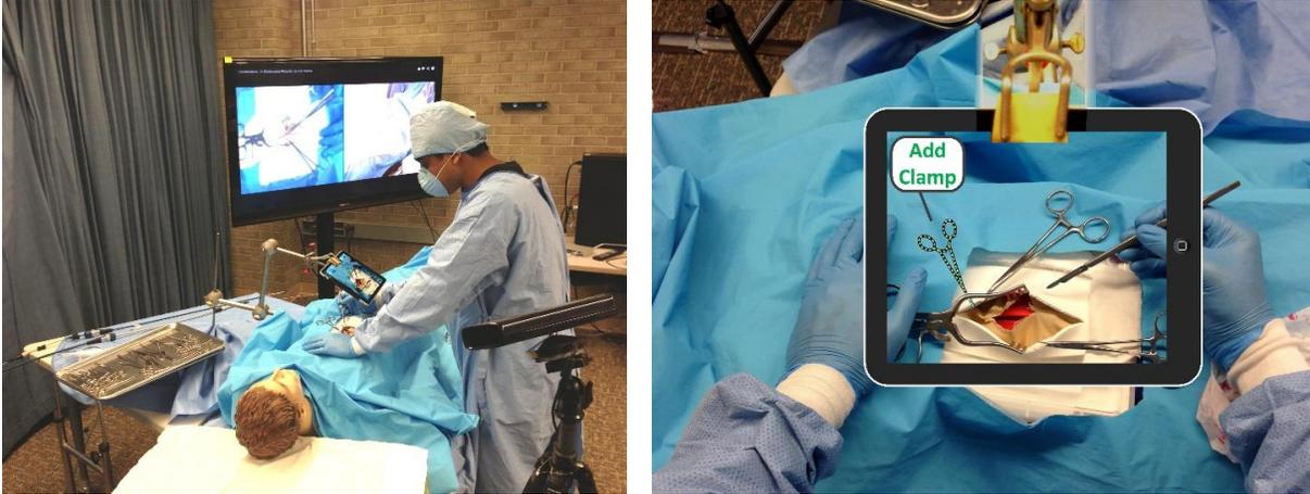
Figure 1: Concept illustration of augmented reality transparent display telementoring approach: overall view of trainee site (left), and trainee view (right).
